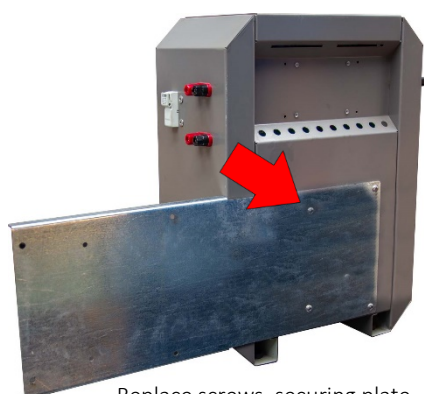
Replace screws, securing plate
